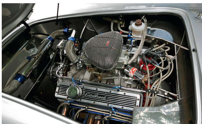
Above top: This recently built customer car was the last one completed in the cramped London premises. If the timing works out, this car will be at our Kitfest at Castle Combe on 19 July. Above left: The recommended Chevy 5.7-litre small-block engine starts at 250bhp/350lbs.ft, rising to twice that with frisky cams, fancy pistons and heads and more and bigger carb barrels. Above right: The interior of the freshly-finished Cobretti still has the Jaguar steering wheel for passing the IVA test. Black leather seats will only look better as they get comfortable with use. Below: There's a big Nitrous bottle in the boot, so there might be 400bhp on tap. Oo-er Missus!
